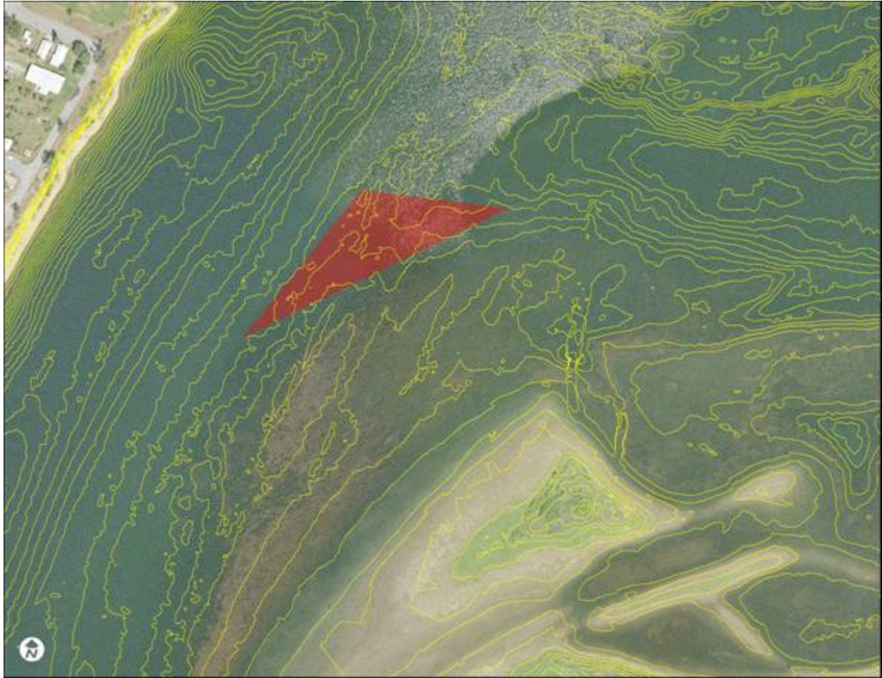
Figure 3.2-2. Proposed location of macrophyte bottom barrier in the Metaline Pool, across from the Town of Metaline (PRM 28.7). Area shown in red indicates the location within which bottom barrier could be installed.
