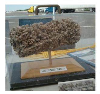
This 2" ABS pipe was submerged in Lake Mead for 6 months. This pipe, located at the Highway 2 inspection station demonstrates:
