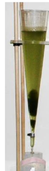
Raw water sample collected using a 64 micron plankton tow
